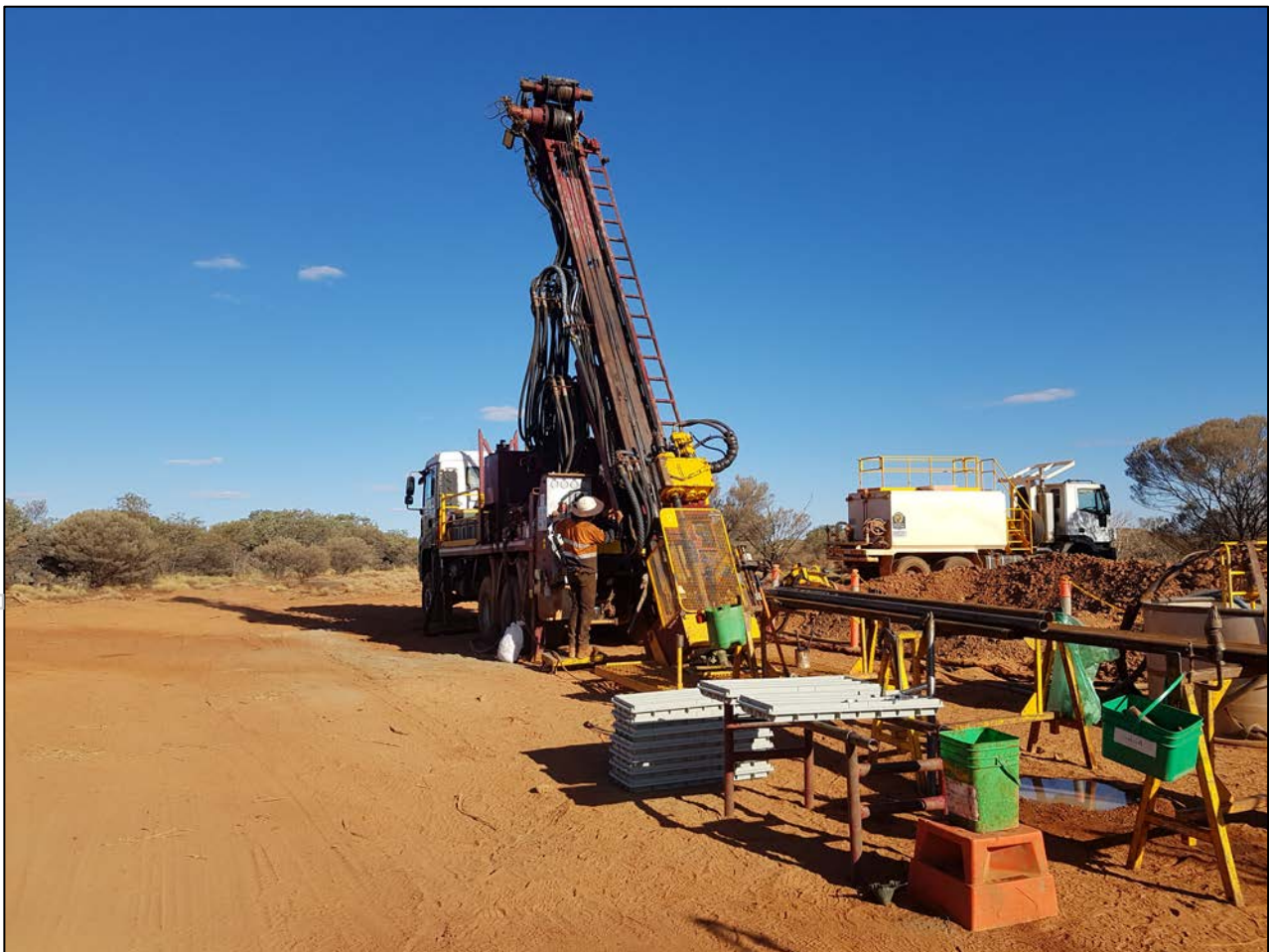
Image 1: Diamond drilling testing three key lode structures in the PHB Corridor, drill hole VHBRC0006
